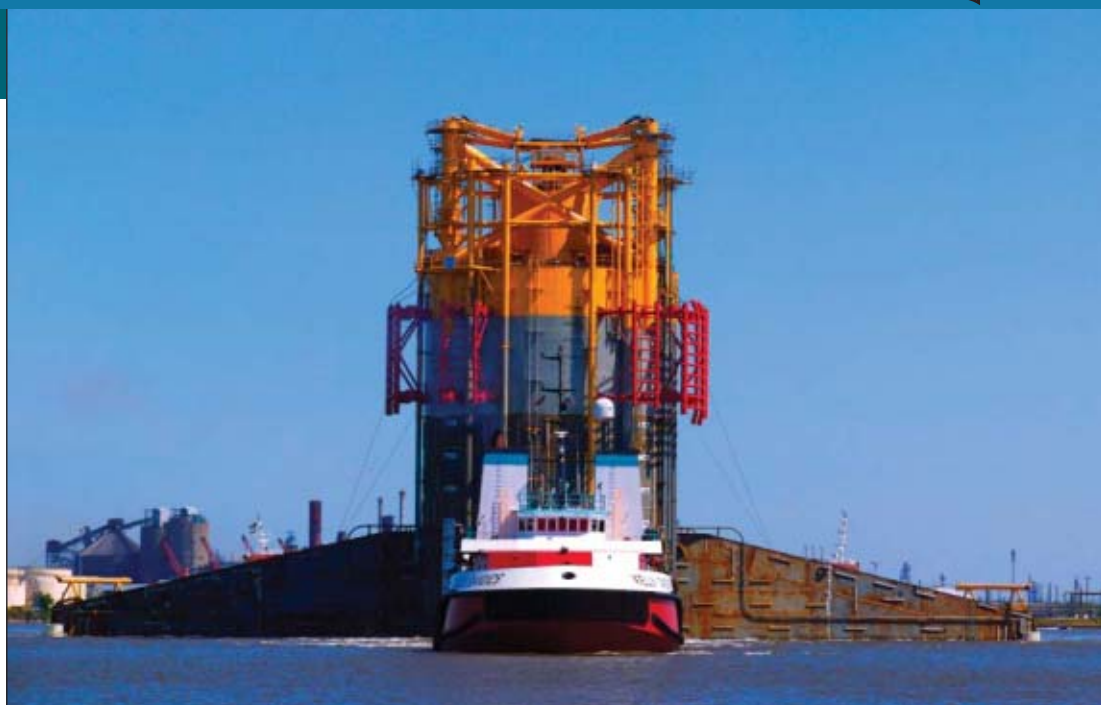
The Kelly Candies, one of three tugs, moves the Neptune TLP hull from Signal International LLC's dry dock in Port Arthur, Tex., for installation on Green Canyon Block 613 in the Gulf of Mexico. Photo from BHP Billiton Petroleum (Americas) Inc.
