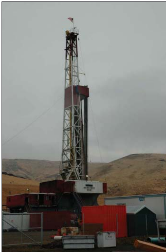
DHS Drilling Co.'s Rig 7 was mobilized from Wyoming to drill the sedimentary sections underlying the basalts in the second and third EnCana wells (Fig. 4; photo by Nina M. Rach).
